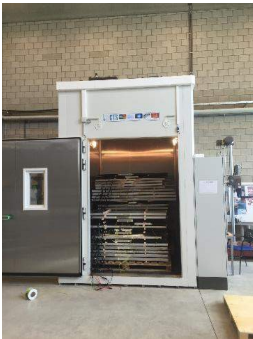
Figure 5: The climate chamber with the PV modules stacked for the PID stress test.
